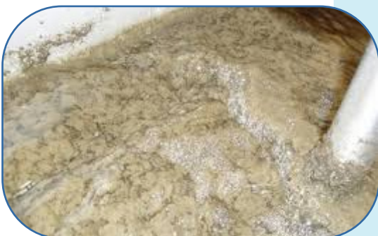
COAGULATED SOLIDS FLOAT ON TOP OF WASTEWATER
