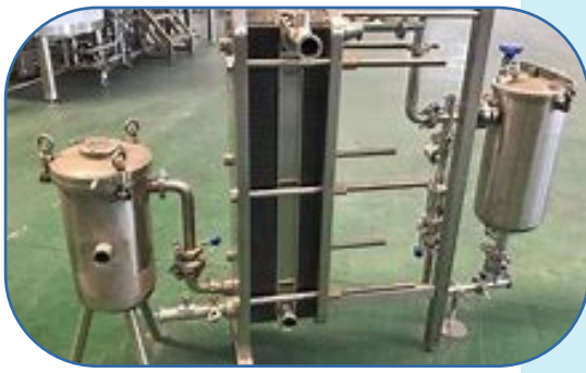
AUTOMATED BREWERY COOLING WATER SYSTEM
